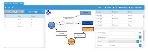
Fig. 1: The RMLEditor with the *Input Panel* on the left, the *Modeling Panel* in the center and the *Results Panel* on the right
